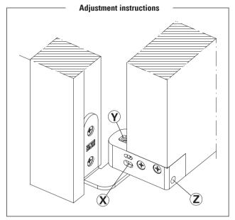
**Horizontal adjustment:** adjust screw «X», using a 4mm Allen key to obtain a  $\pm$  1.5mm adjustment.
