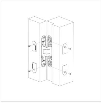
Screw the small cover plates onto the frame and door part with the enclosed, self-tapping screws.
