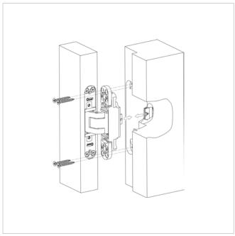
Establish the plug connection in the frame part – depending on adapter version used – and fix the frame part corresponding to frame type.
