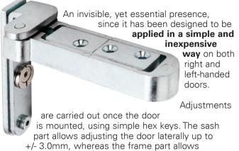
adjusting the depth by +/- 1.5mm.
